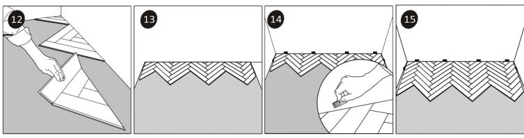
12. Install the starting triangles Connect the cut starting panels to form triangular shapes, one by one. Start installing the triangles from the left corner. It is recommended to use glue to fix the smallest parts of the triangles into place by applying a small quantity of glue inside the groove.
