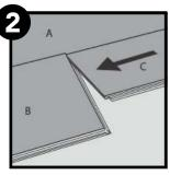
**Figures 1 & 2** - Place plank "A" against the wall. Continue by engaging plank "B" and "C" onto plank "A". When engaging plank"C" please assure the end joint of plank "C" is aligned to the end joint of plank "B". Please see Figures 1 and 2 for guidance.
