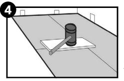
**Figure 4** - Use a tapping block and a hard mallet along both short ends to engage the planks. Place the tapping block over both short ends and tap it with the mallet until the ends are fully engaged. Please be careful not to damage the profile or edges while engaging the planks. Test each plank before proceeding to the next row to make sure they are fully engaged. Please refer to the installation instructions for detailed steps.
