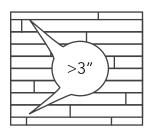
Before starting, carefully measure the length and the width of the room to plan a precise layout to achieve a balanced appearance of the floor. This is very important when installing typical plank decors. This will also ensure that you won't end up with the last row being too narrow. If the last row will be less than 3" (8cm), the installation will be easier and better if you reduce the width of the planks of the first row.
