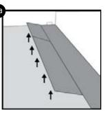
Disassemble the panels by lifting the short ends upward and disengage from the rest.
