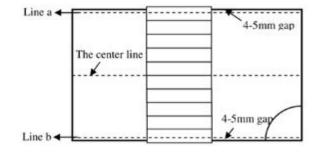
• Measure the width of the room at the front, middle and back and divide the widths of each measurement by the width of a plank. If the remainder is less than half the plank width, then the planks on your starter row should be narrowed to make the last row approximately half the plank. The width of the last row of planks should be approximately the same width as the first row of planks.
