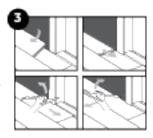
Do not fill or cover the expansion joints with silicone or other kit.
