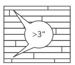
Before starting, carefully measure the length and the width of the room to plan a precise layout to achieve a balanced appearance of the floor. This is very important when installing typical plank decors. This will also ensure that you won't end up with the last row being too narrow. If the last row will be less than 3" (8cm), the installation will be easier and better if you reduce the width of the planks of the first row.
