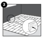
Inspect the final surface of the installed floor. Install vinyl skirtings against the wall but never attach the skirting to the floor itself. This method allows the floor to expand and/or contract under the skirting-board.
